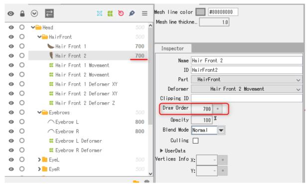
The value output by csmGetDrawableDrawOrders is the value in Cubism Editor's inspector. Calculation of drawing order group is not related.
