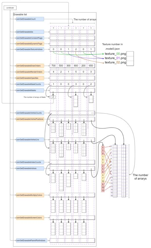
In loading Drawable, preparation for attribute of the render such as registration to the graphics API or generation structure for drawing order sorting will be getting done.
