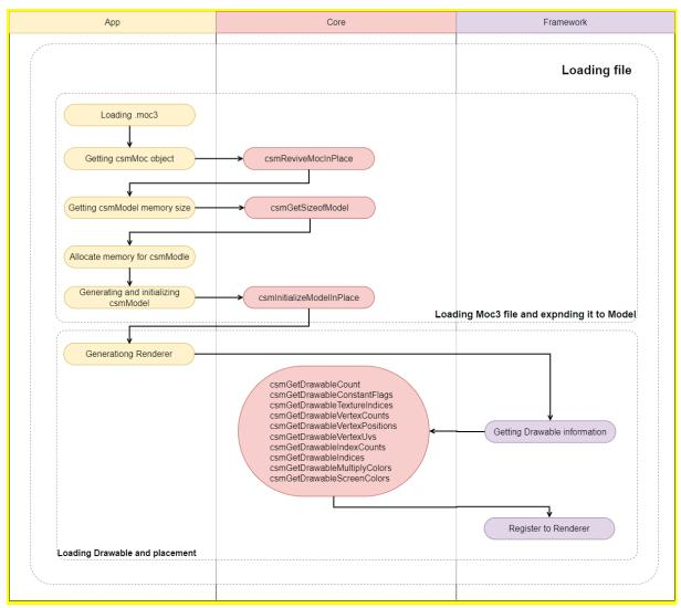
Yellow node shows Application, purple node means a segment Framework should process. Nodes with arrow to the Core indicate calls to API of the Core.
