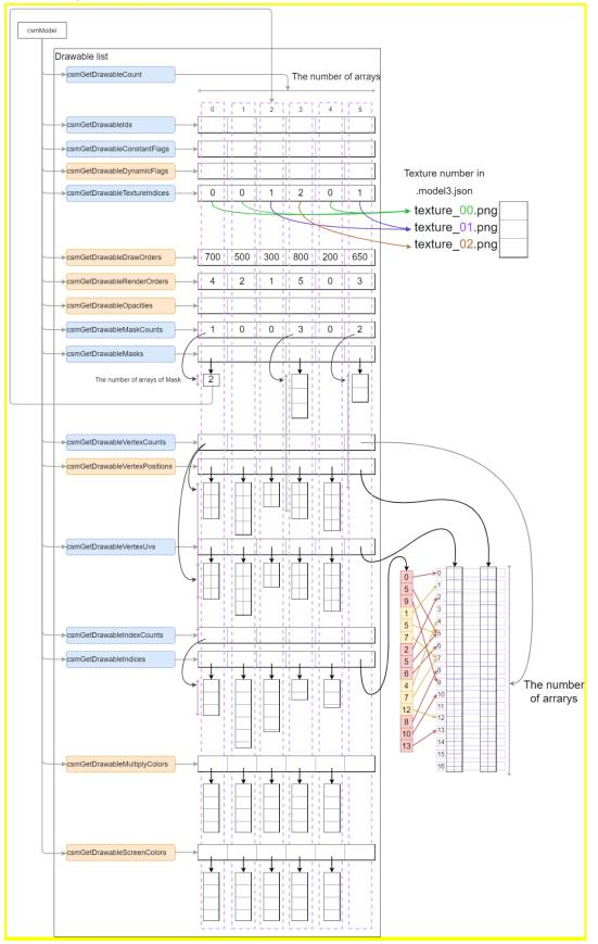
In loading Drawable, preparation for attribute of the render such as registration to the graphics API or generation structure for drawing order sorting will be getting done.
